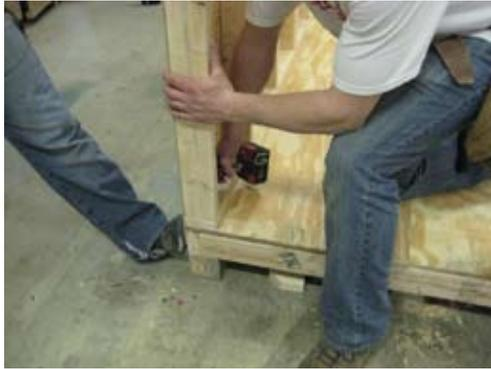
Push wall in and make sure it is flush on end. Secure with 2 1/2" screw.
