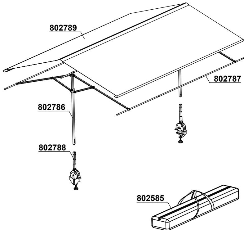
**1. ATTACH QUICK CLAMP BRACKETS, 1 ON EACH SIDE**
